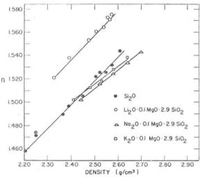
Fig. 1. The refractive indices refer to the sodium D line for silica glass and to white radiation for the other glasses. Each point represents an uncertainty of  $\pm 0.005$  index of refraction units and  $\pm 0.01$ g per cm<sup>3</sup> density units. Compositions are expressed as molar
